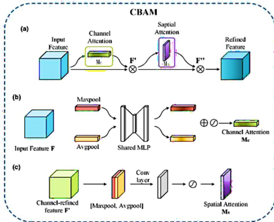
Fig. 5 Structures of the CBAM: (a) Overall structure of CBAM module; (b) Attention channel module structure; and (c) Attention spatial module structure (Niu et al., 2021).
