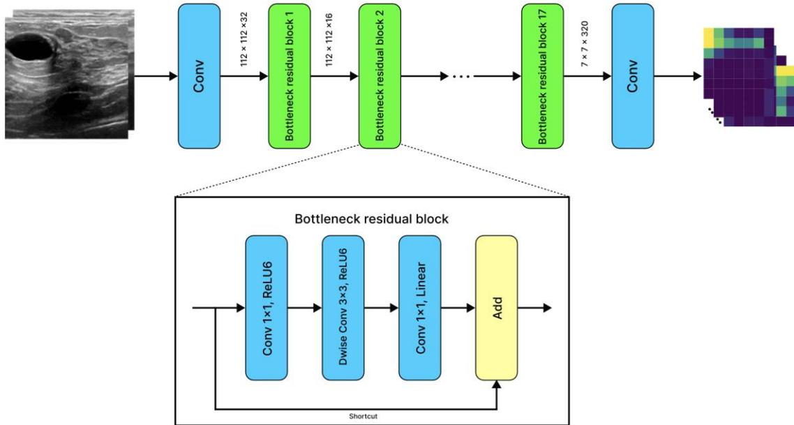
Fig. 4. The architecture of the MobileNetV2 network (Sandler et al., 2018).
