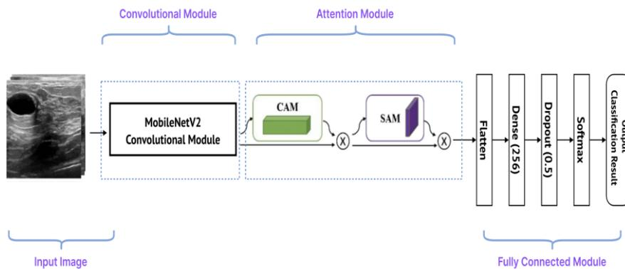
Fig. 7. Proposed architecture of the MobileNetV2-CBAM.
