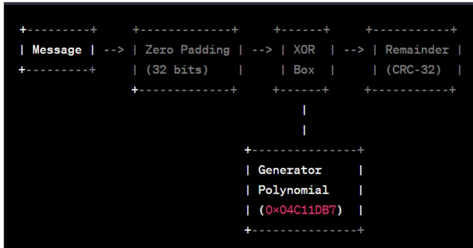
Fig. 4. Block Diagram of CRC 32.
