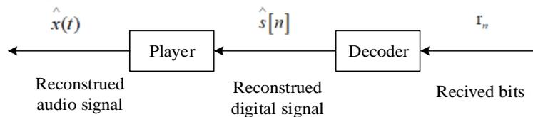
Fig. 3. Reconstruction process of Audio Signal to Bit Received.
