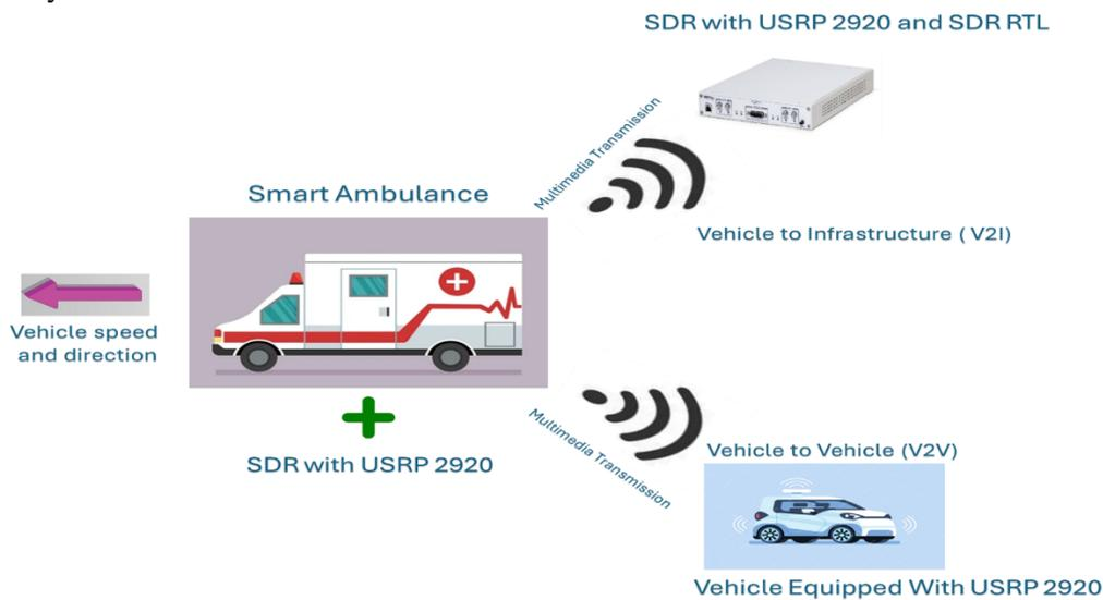
Fig. 1. Proposed Smart Ambulance with software-defined radio (SDR).
