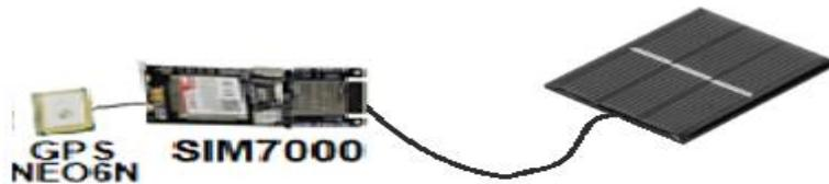
Fig. 3. SM7000G connected to solar cell
