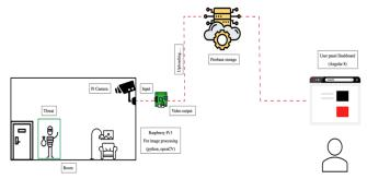
Fig. 2. The overall proposed system design
