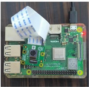
Fig. 5. The utilised Raspberry Pi-3 with the compatible camera
