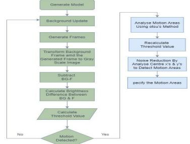
Fig. 8. Flowchart for the overall proposed algorithm.
