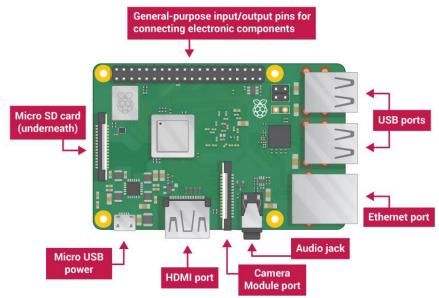
Fig. 1. Raspberry Pi 3 structure.
